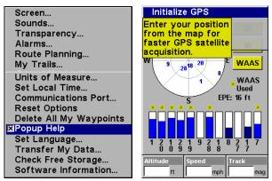
System Setup Menu (left) with Pop-up Help command highlighted. The second example (right) shows the Pop-up Help message for the Initialize GPS command, located on the Status Page menu.
